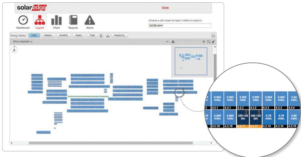
The SolarEdge monitoring server provides full visibility of system performance & remote troubleshooting for effective O&M management. The zoom-in provides module-level energy production and pinpoints underperforming modules, thus allowing the Directorate of the IAOSB to proactively manage its solar assets. This screenshot shows daily energy production.
