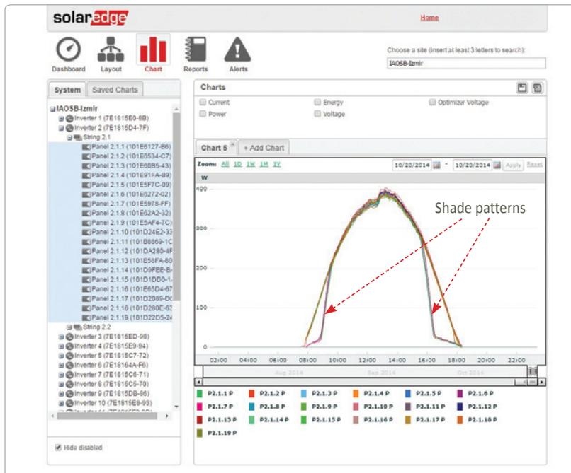
The chart view from the SolarEdge monitoring server shows the performance of individual modules. As illustrated in the graph, the power of each module is optimal and independent of other modules in the same string in order to provide increased energy production throughout the system lifetime.
