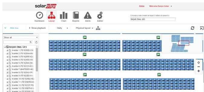
The layout view from the SolarEdge monitoring portal shows the performance of individual modules and their physical location. The graph illustrates the power of each module and the slight inherent mismatch between modules. Mismatch losses are eliminated due to the module level optimization
