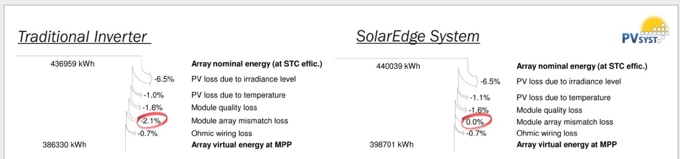
Energy output simulation with Pvsyst, independent design & simulation software, showing a **2.1% mismatch loss for the traditional inverter system** and **0% mismatch loss for the SolarEdge system**.
