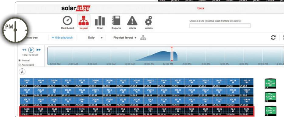
Screenshots from the cloud-based monitoring portal showing the physical layout and the module-level production at specific times. In the afternoons, the bottom row of panels, outlined in red, is darker, signifying a decrease in energy production caused by inter-row shading. The shaded modules, installed in the same string as the non-shaded modules, do not negatively impact production of other modules in the same string.
