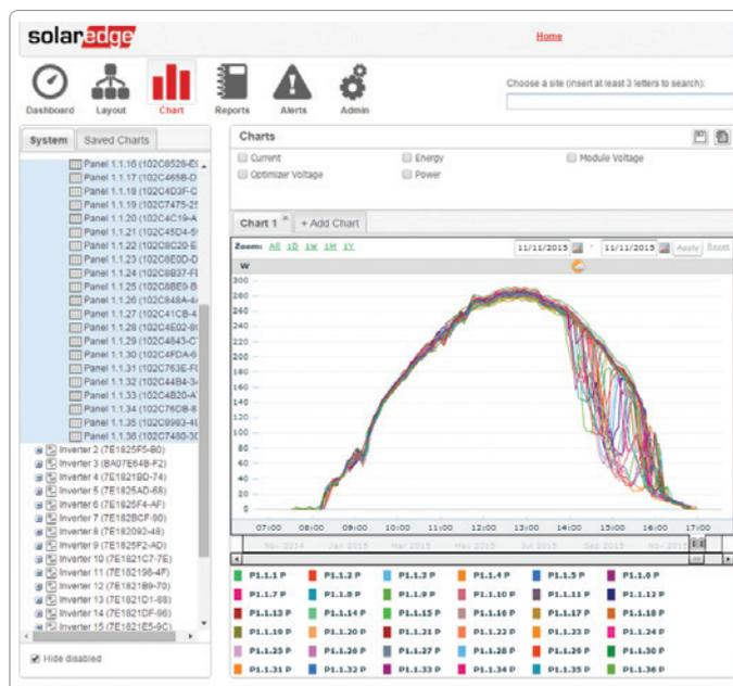
The chart view from the SolarEdge monitoring portal shows the performance of individual modules. This graph illustrates that the power of each module is optimal and independent of other modules in the same string. The dips show the effects of inter-row shading.
