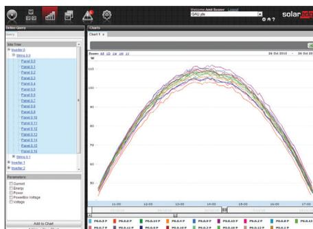
*Screenshot: Individual module power curves plotted by the SolarEdge Monitoring Portal. Despite noticeable mismatch between modules, weaker modules do not limit the performance of more powerful modules in that string.*
